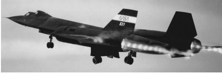
Figure 1.22 SR-71B with shock diamonds in the exhaust (Courtesy of NASA.)
