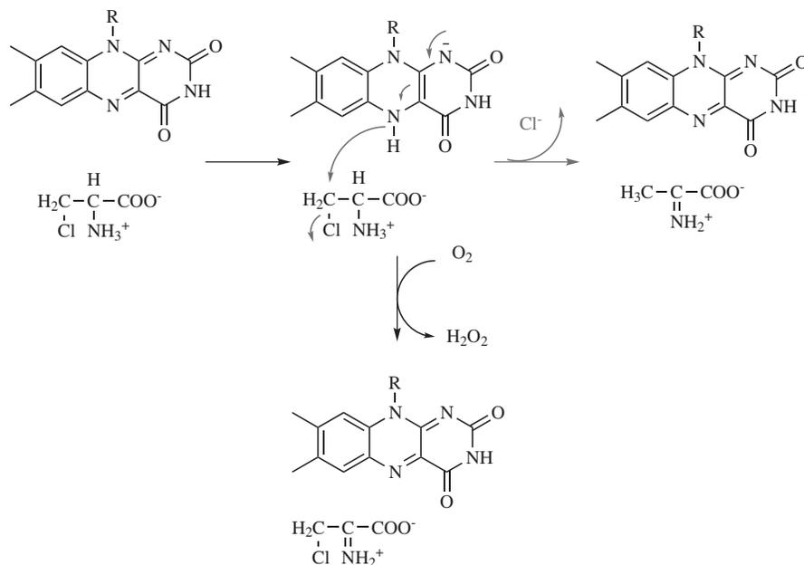
**FIGURE 1.31** Proposed mechanism for the oxygen concentration-dependent amine oxidation versus HCl elimination in DAAO-mediated reactions.
