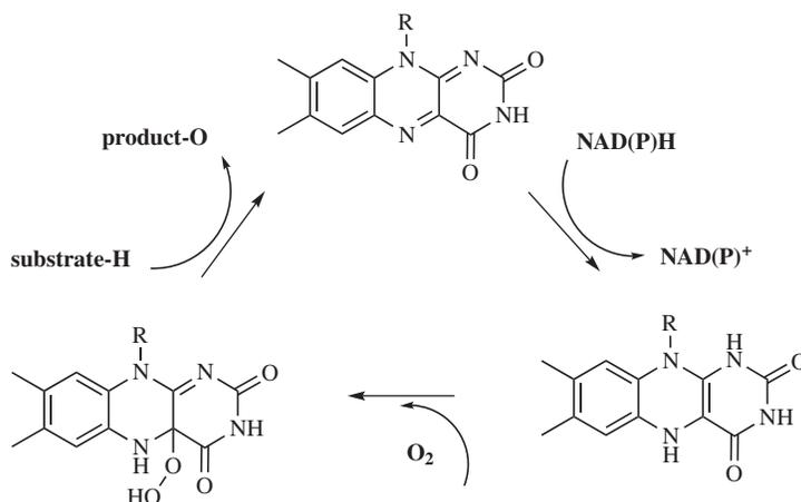
**FIGURE 1.10** Schematic oxygenation mechanism for flavin-dependent monooxygenases.
