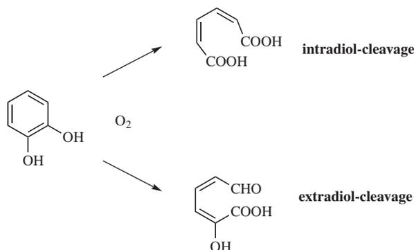
**FIGURE 1.15** Intradiol vs. extradiol cleavage reaction mediated by catechol dioxygenase.
