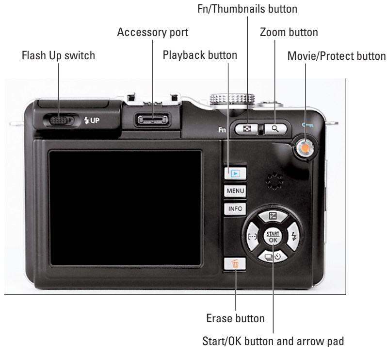
Figure 1-2: Use the Start/OK button and surrounding arrow keys to navigate menus and adjust picture-taking settings.
