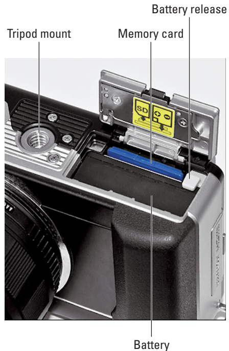
Figure 1-4: The battery and memory card share an apartment next to the tripod mount.
