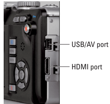
Figure 1-3: Open the cover on the right side of the camera to reveal ports for connecting the camera to a computer or TV.
