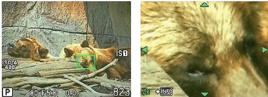
Figure 1-24: Press the Zoom button to magnify the display for a close-up look at your subject.
