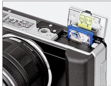
Figure 1-11: Insert the card with the label facing the front of the camera.
