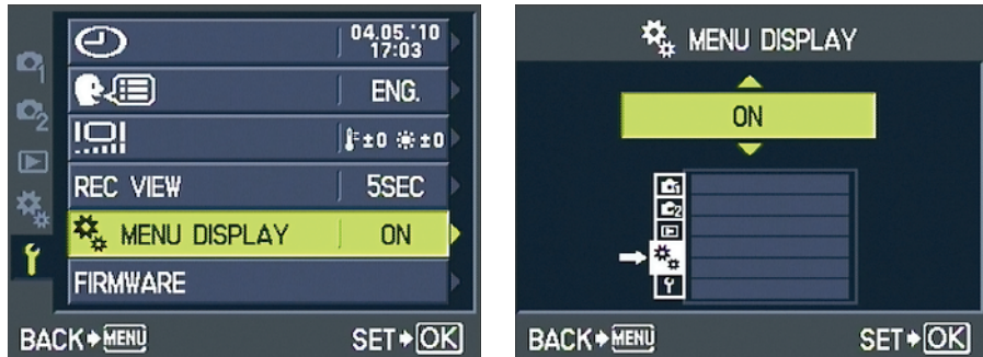
Figure 1-15: To display the hidden menu, choose this setting on the Setup menu.
