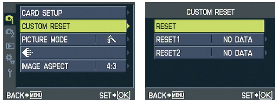
Figure 1-38: To access the Custom Reset option, first set the Mode dial to P, A, S, or M.
