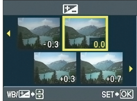
Figure 1-23: The Multi View display enables you to preview the effects of four Exposure Compensation settings side-by-side.
