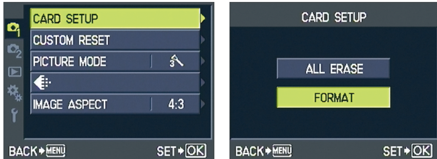
Figure 1-12: Format a memory card through the Card Setup option on Shooting Menu 1.
