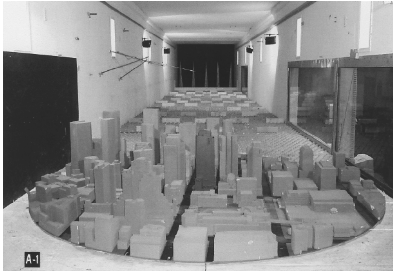
FIGURE 1.16 Scale model of the St. Regis Hotel and Residences and surroundings in a wind tunnel. CPP Wind Engineering
