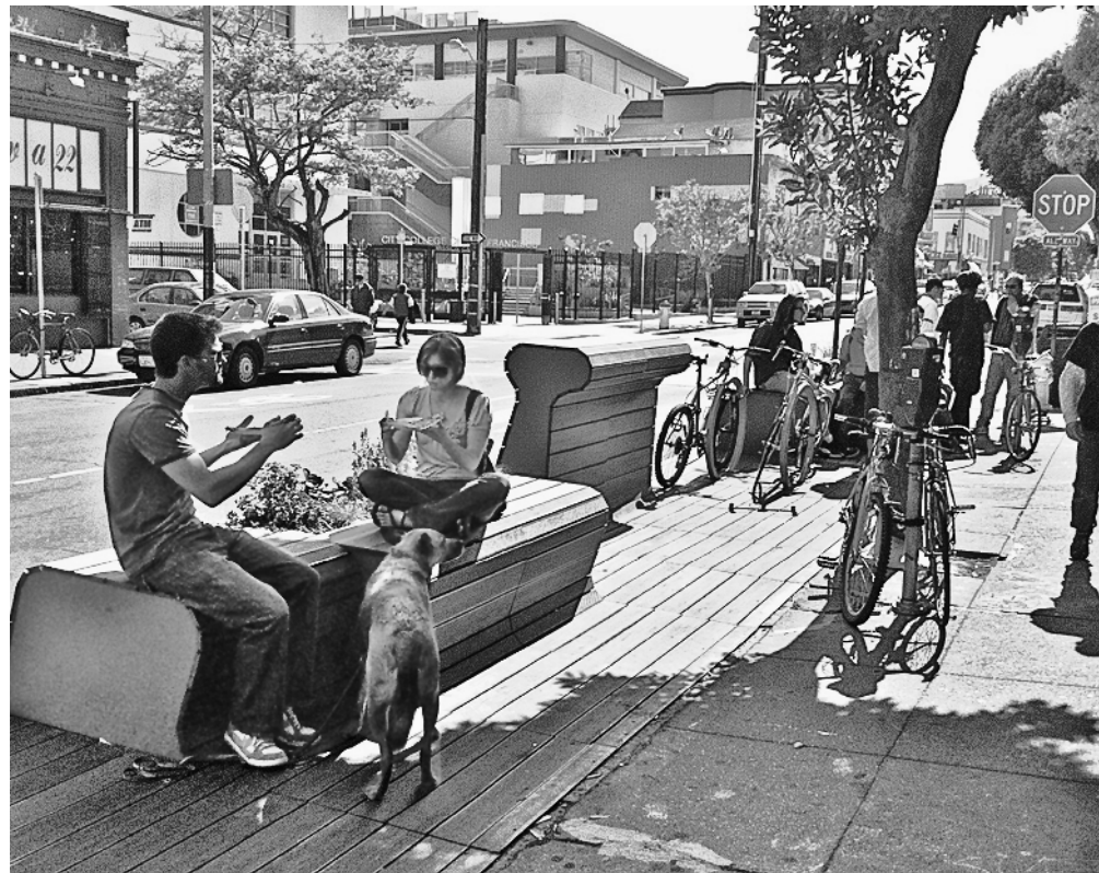
Figure 1-18 This parklet is a temporary sidewalk extension with a modular design that fits in the width of a parking lane. Photo: Rebar Copyright © 2010 by Rebar Group, Inc. Walklet is a registered trademark of Rebar Group, Inc. Used with permission.
