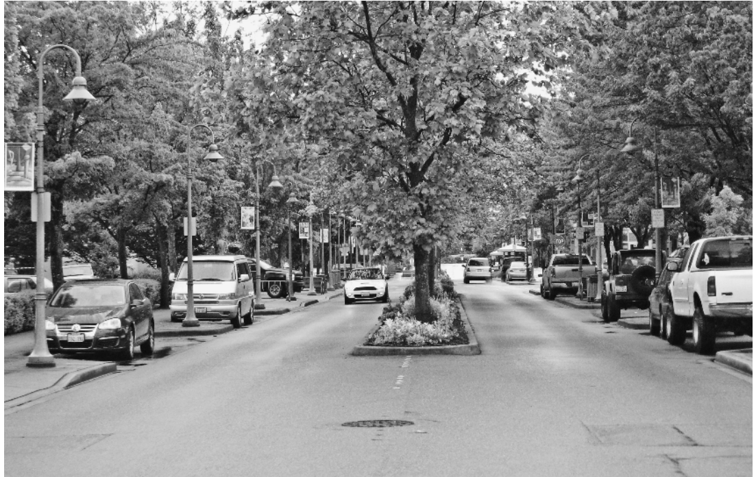
Figure 1-6 Trees in the street and the median create a volume of space that deemphasizes the travel lanes. In this case, the trees compensate for the lack of buildings along the street edge.
