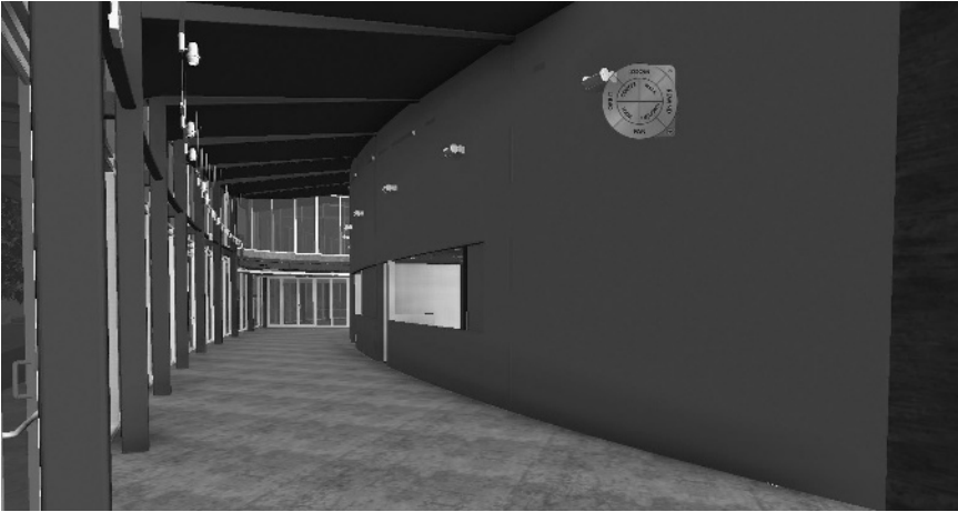
Figure 1.8 BIM showing how an owner can view the hallway of a building.
