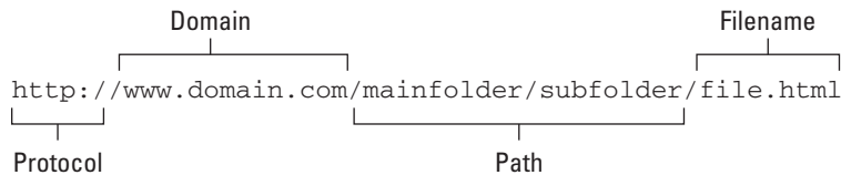
Figure 1-3: The components of a URL help it define an exact location for a file on the Web.
