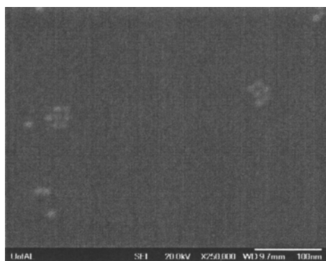
Figure 1. SEM image of gold nanoparticles dispersed on silicon substrates.
