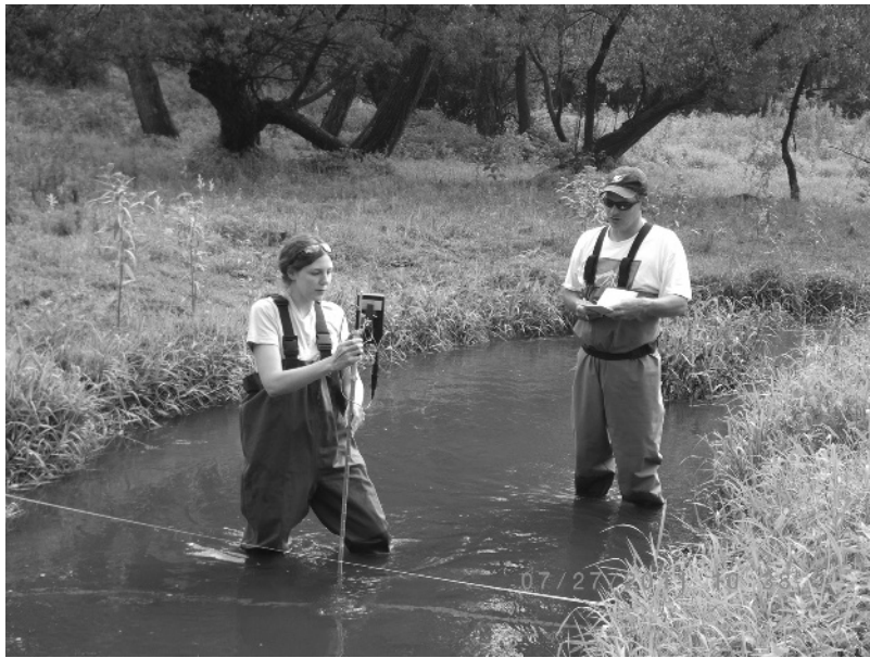
PHOTO 3. Students measuring streamflow with a current meter (Photograph by Lucas Bistodeau) (For a color version of this photo, see the color plate section)
