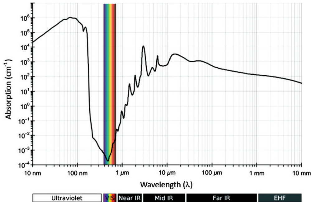
Figure 1.2 Human sensitivity to light Visible light corresponds closely to the wavelengths of minimum water absorbance on the electromagnetic spectrum. See also Chapter 2, Section 2.5. Since our eyes are composed largely of water, it is advisable to use a heat filter (e.g. Schott KG5) in the light path to cut out any absorption of infrared light. Source: Adapted from Kebes at English Wikipedia under the terms of the Creative Commons Attribution licence, CC BY-SA 3.0 ( http://creativecommons.org/licenses/by-sa/3.0 ).
