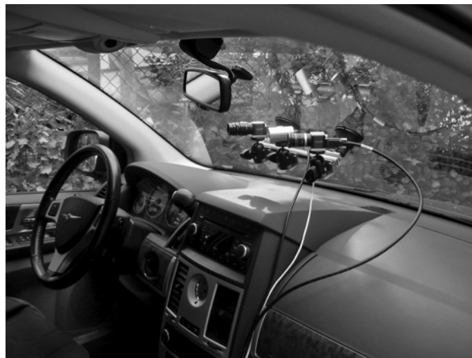
Figure 1.1 System of cameras mounted in a car. The cameras can observe a driver to monitor his/her state. Cameras can also observe the front of a car for pedestrian detection or road sign recognition. Such vision modules will probably soon become standard equipment, being a part of the on-board Driver Assisting System of a car.
