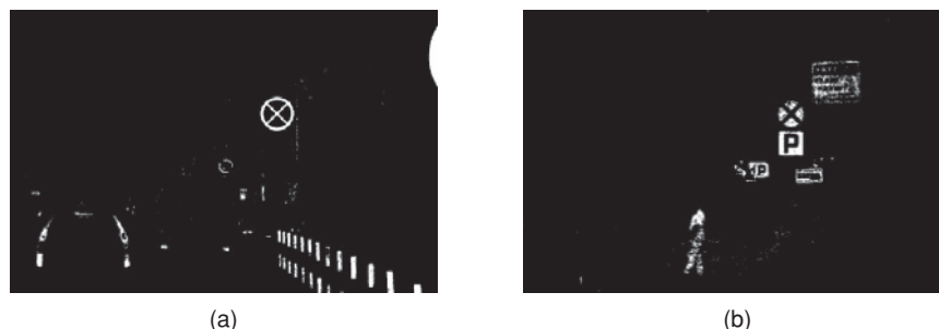
Figure 1.4 Segmentation of image in Figure 1.2. Red (a), blue color segmentation (b).
