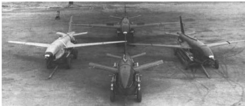
Figure 1.6 Several variations of the Ryan Model 147 unmanned reconnaissance drone used in the 1960s and 1970s [5]
