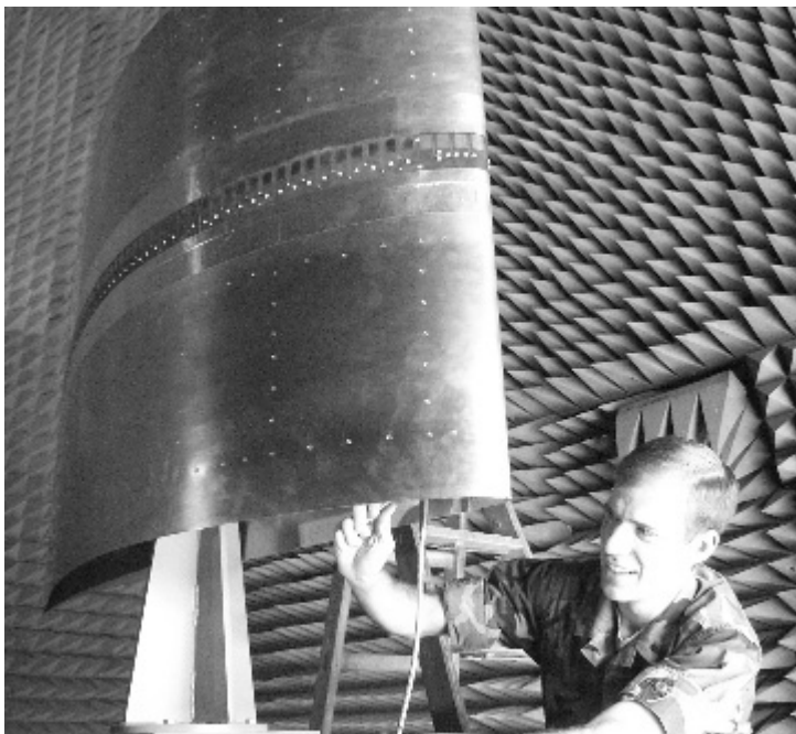
Figure 1.3. A microstrip array conformal to a wing profile in the test chamber. See also color insert, Figure 1. (Courtesy of Air Force Research Lab./Antenna Technology Branch, Hanscom AFB, USA.)
