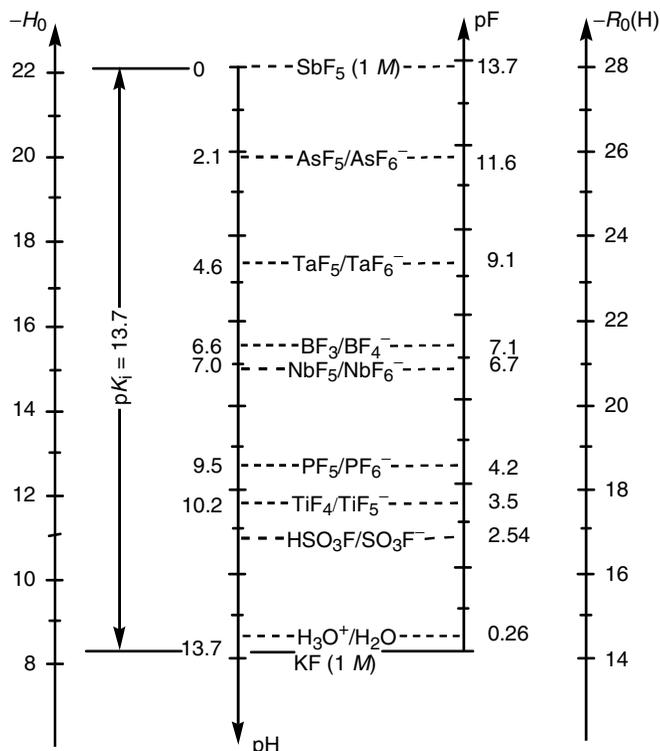
**Figure 1.9.** Relative strength of some strong Lewis acids as measured in HF on the pH scale by electrochemical titration.<sup>48</sup>
