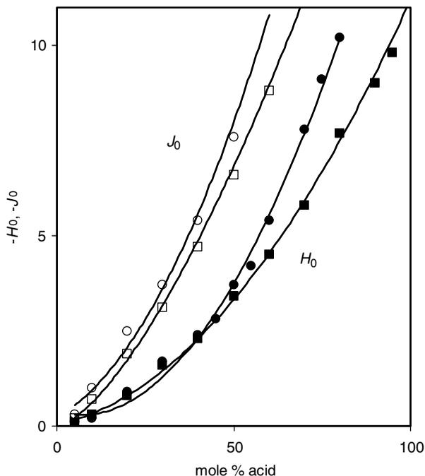
**Figure 1.1.**  $H_0$  and  $J_0$  functions for  $\text{H}_2\text{SO}_4\text{-H}_2\text{O}$  and  $\text{HClO}_4\text{-H}_2\text{O}$  systems.  $\text{HClO}_4$ :  $\circ$ , ref. 11;  $\bullet$ , ref. 13;  $\text{H}_2\text{SO}_4$ :  $\square$ , ref. 12;  $\blacksquare$ , ref. 14.
