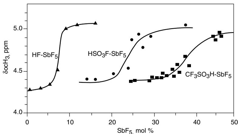
**Figure 1.7.** Protonation curves of indicator **3** in the superacid systems (from left to right)  $\text{HF-SbF}_5$ ,  $\text{HSO}_3\text{F-SbF}_5$ , and  $\text{CF}_3\text{SO}_3\text{H-SbF}_5$ .<sup>22</sup>
