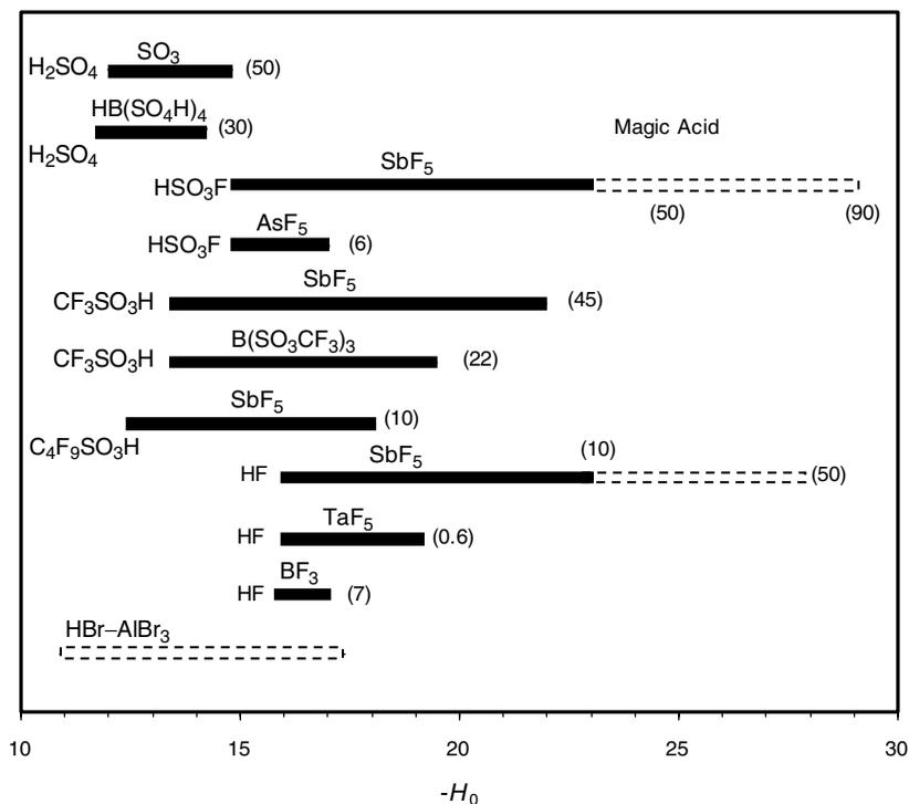
**Figure 1.3.** Acidity ranges for the most common superacids. The solid and open bars are measured using indicators; the broken bar is estimated by kinetic measurements; numbers in parentheses indicate mol% Lewis acid.
