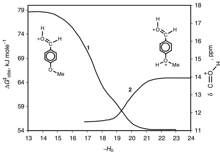
**Figure 1.8.** Complementarity of NMR methods in determining the variation of the acidity with the ionization of the indicator.<sup>46</sup> Curve 1: line-shape analysis; curve 2: chemical shift measurement.
