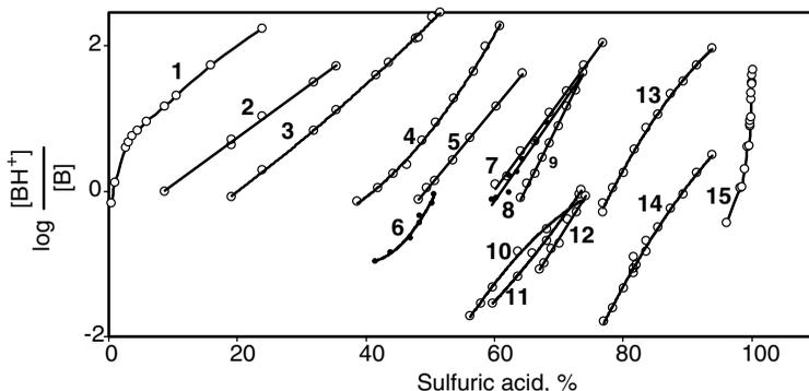
**Figure 1.4.** The ionization ratio as measured for a series of indicators in the 0–100%  $\text{H}_2\text{SO}_4$ – $\text{H}_2\text{O}$  system.<sup>8</sup>
