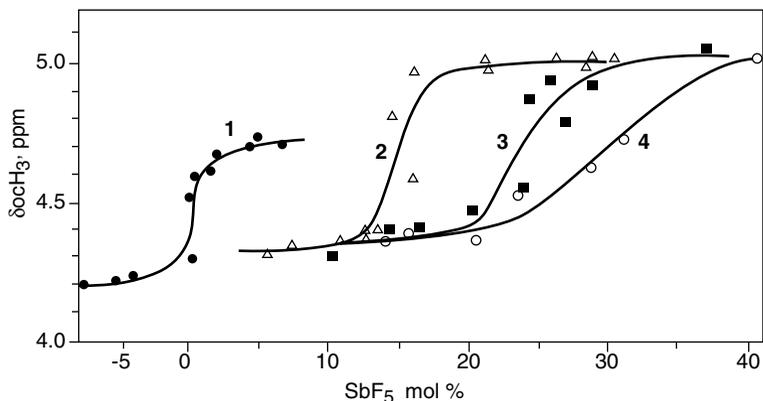
**Figure 1.6.** Protonation curves of indicators **1–4** in the  $\text{HSO}_3\text{F-SbF}_5$  system.<sup>22</sup>
