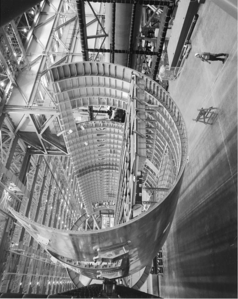
**Figure 1.15** Fuselage of a Boeing 777 under construction. (Courtesy of the Boeing Company.)
