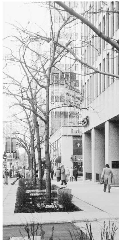
FIGURE 1.4-3 (a) Planting strips help organize and separate street furniture from the pedestrian path. (b) Rest areas may be integrated with planting strips to provide convenient stopping places outside the circulation path.
