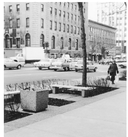
FIGURE 1.4-9 The textured surface around the planter and the bench serves as a warning to those with visual impairments.
