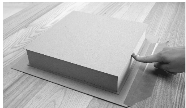
Figure 1.16 Floor or roof diaphragm stabilizing the top edge of a loaded wall.
