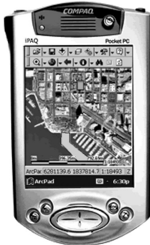
Figure 1.10 Handheld Computer Running ArcPad Software. Source: ESRI Inc.
