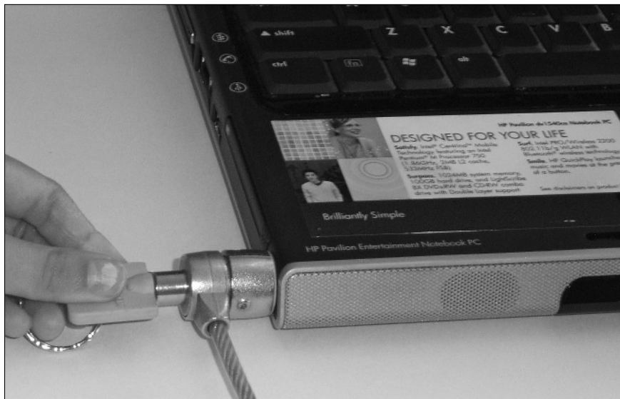
Figure 1-6: A lockdown cable is used to secure computer equipment to a desk.
