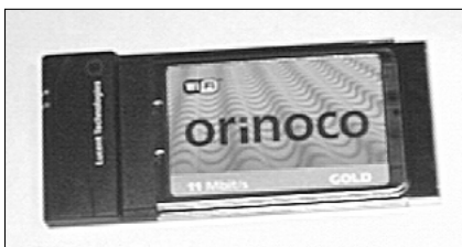
Figure 1-4: A PC Card wireless network interface adapter.
