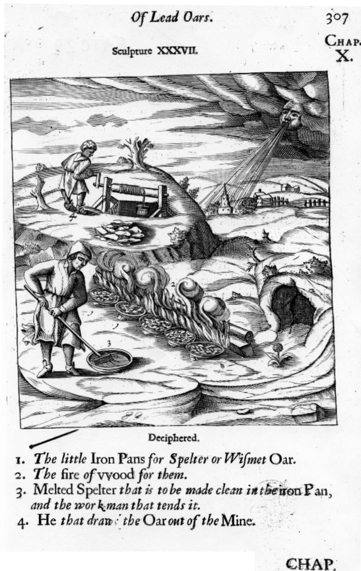
FIGURE 29. ■ Smelting of bismuth ore in the open wind from Pettus' 1683 Fleta Minor . Compare this figure with the corresponding one (Figure 15) in the 1736 edition (i.e., the original 1574 edition), and you will note that costumes have been updated by a century while the apparatus remains unchanged.
