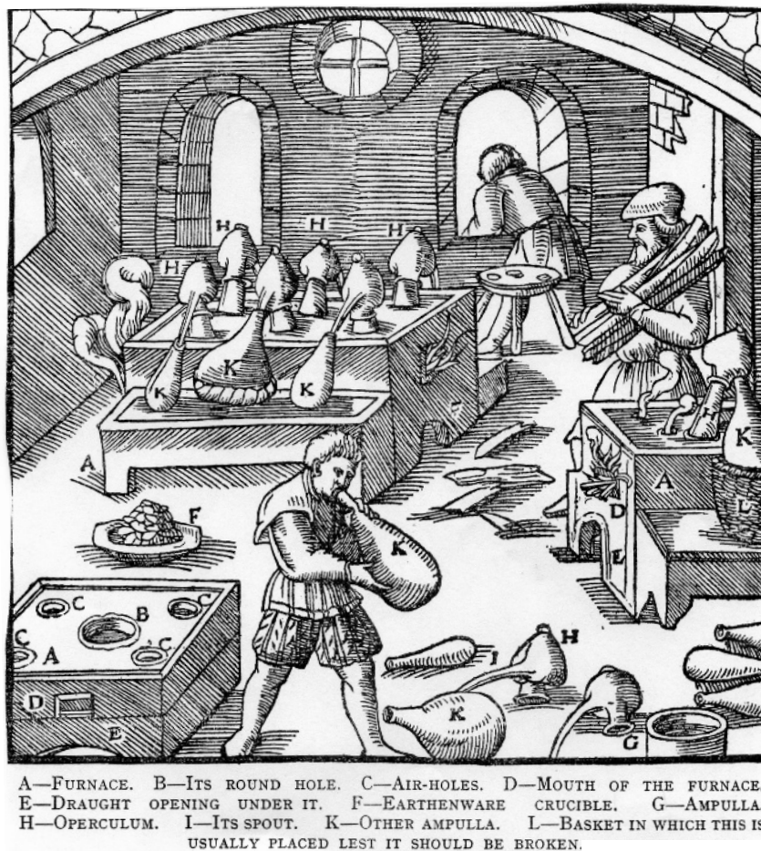
FIGURE 21. ■ Distillation of aqua valens (“powerful water”), a general term used by Agricola to describe powerful acids such as aqua fortis (nitric acid) and aqua regia (hydrochloric acid/nitric acid, 3 : 1), depicted in the 1912 Hoover translation of Agricola’s 1556 De Re Metallica .
