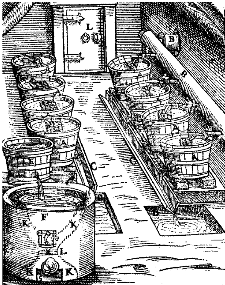
FIGURE 16. ■ Steps in the leaching and concentration (by boiling) of saltpetre obtained from old sheep dung (Ercker, see Figure 5).
