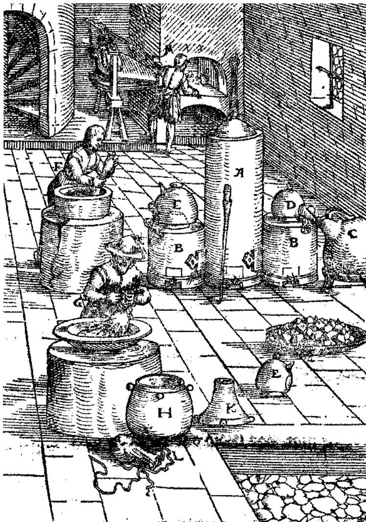
FIGURE 11. ■ Use of mercury to dissolve gold in ore concentrates. The gold amalgam is then heated and mercury distills (Ercker, see Figure 5).
