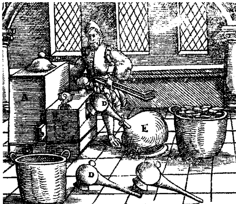
FIGURE 12. ■ Distillation of aqua regia (3:1 HCl/HNO 3 ) (Ercker, see Figure 5). This “kingly water” is capable of dissolving gold. (See essay in Section IX “The Chemistry of Gold is Noble But Not Simple.”)
