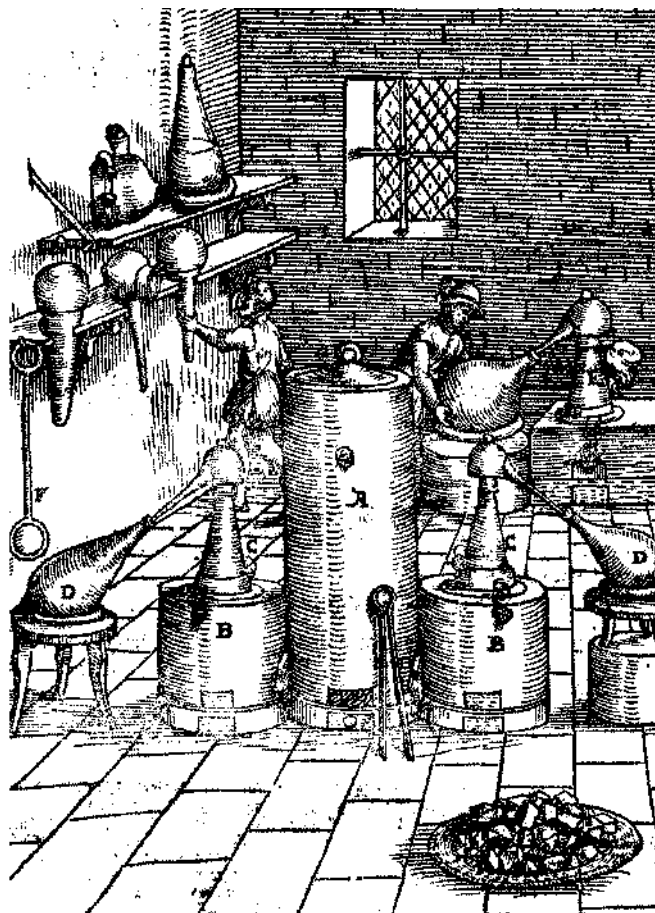
FIGURE 13. ■ The use of “parting acid” (mostly \text{HNO}_3 ) to separate silver from gold. Silver is soluble and gold is not soluble in this acid (Ercker, see Figure 5).
