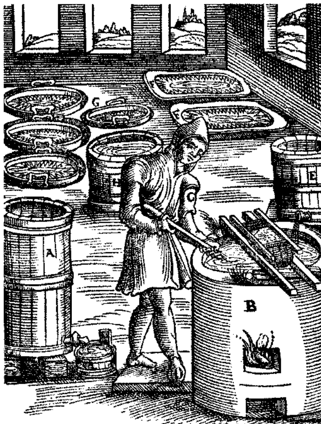
FIGURE 17. ■ Pans and tubs from crystallizing concentrated leachate for saltpetre (see Figure 16). One hundred pounds of the concentrate yields about 70 pounds of saltpetre (Ercker; see Figure 5).
