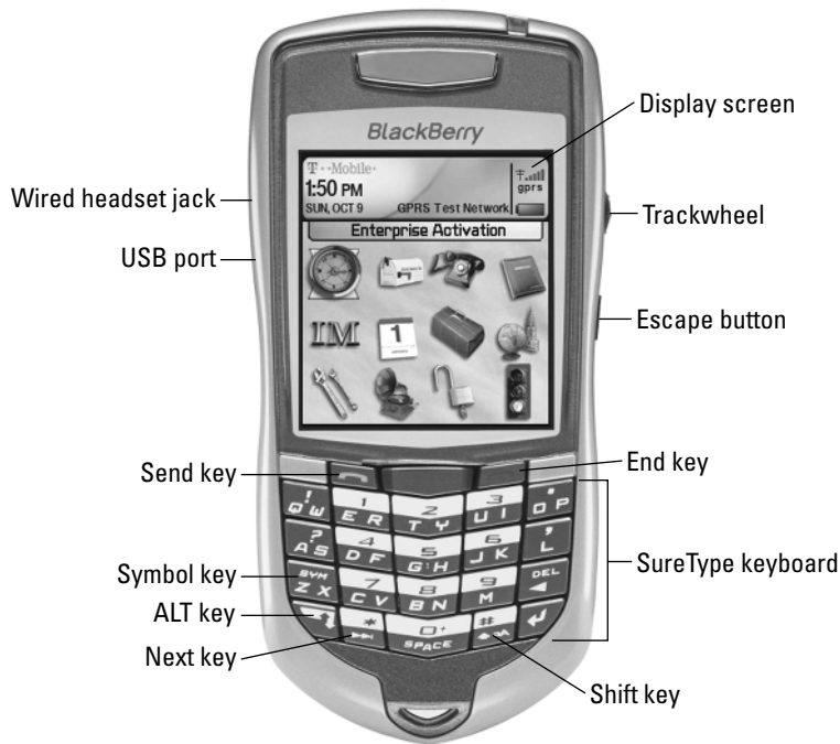
Figure 1-3: Components on a 7100 BlackBerry model.
