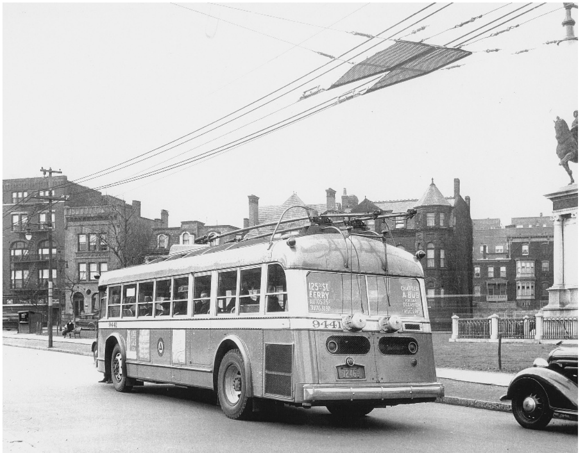
Photo 1.18 Dual-mode electric-ICE bus with automated trolley pole raising, Public Service in New Jersey in 1935 (From the collection of Jeffrey Marinoff)
