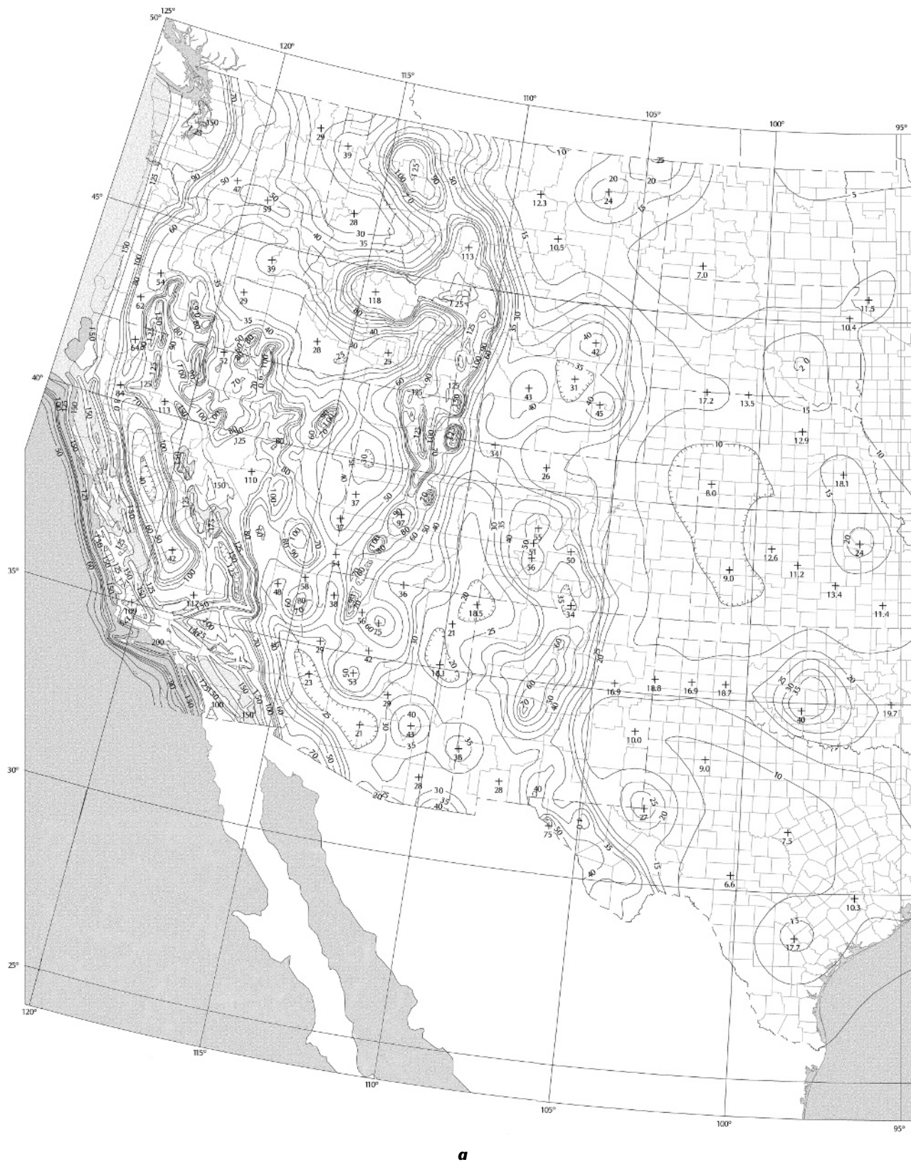
Figs. 1.13a, 1.13b Response acceleration at short periods S_s
