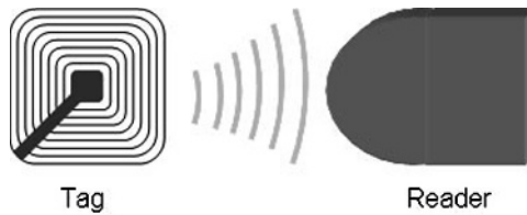
Figure 1-3 Simple RFID system.
