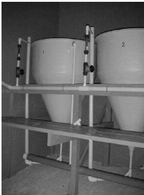
Figure 1.4 Yolk sac larvae incubator.
