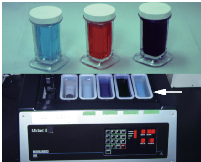
Figure 1.16 Blood film and cytology staining apparatus. Top. Manual staining jars containing Diff-Quick stain. Slides are manually moved from one jar to the next according to the manufacturer's instructions. Bottom. An automated stainer used for higher-throughput situations. Note the mechanical arm that moves a rack of slides (not shown) through the sequence of staining procedure baths (arrow). The stainer may be programmed to control the timing in each bath. Most such machines provide the ability to stain as many as 20–25 slides per cycle.
