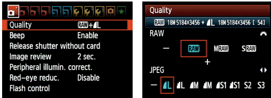
Figure 1-15: Use the multicontroller to navigate menus; press Set to access available settings.
