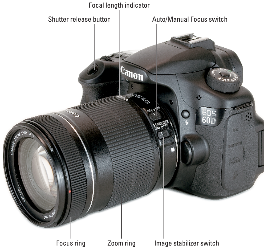
Figure 1-6: The MF and IS controls are generally close together on the lens (which makes them easy to operate).
