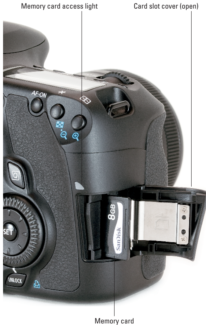
Figure 1-7: Insert the card with the label facing you as you hold the camera.
