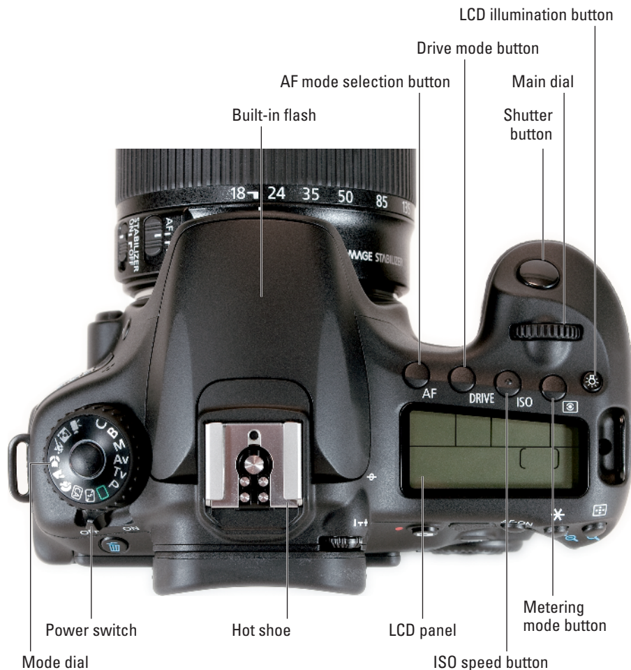
Figure 1-9: The tiny pictures on the Mode dial represent special automatic shooting modes.
