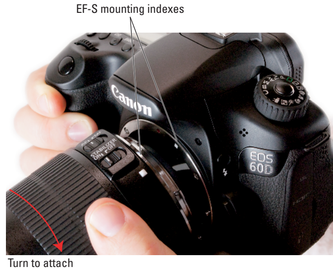
Figure 1-5: Place the lens in the lens mount with the mounting indexes aligned.
