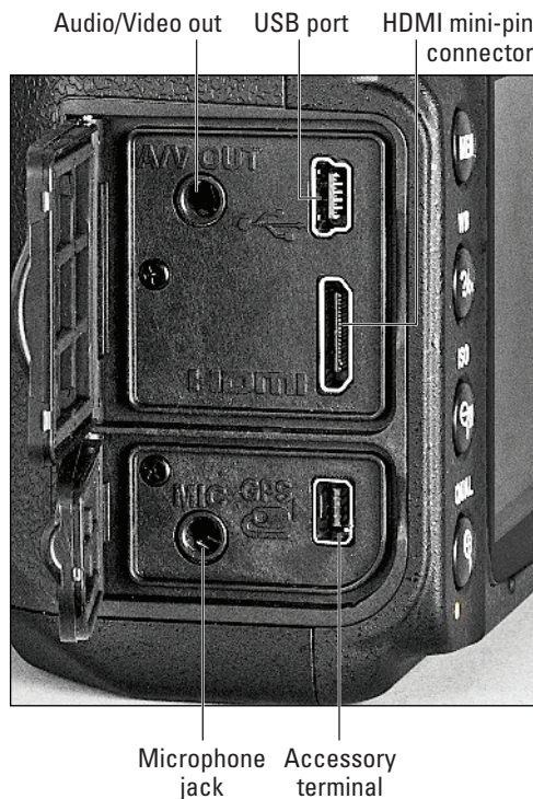
Figure 1-23: You can plug in an external flash cord, remote control, or GPS unit here.
