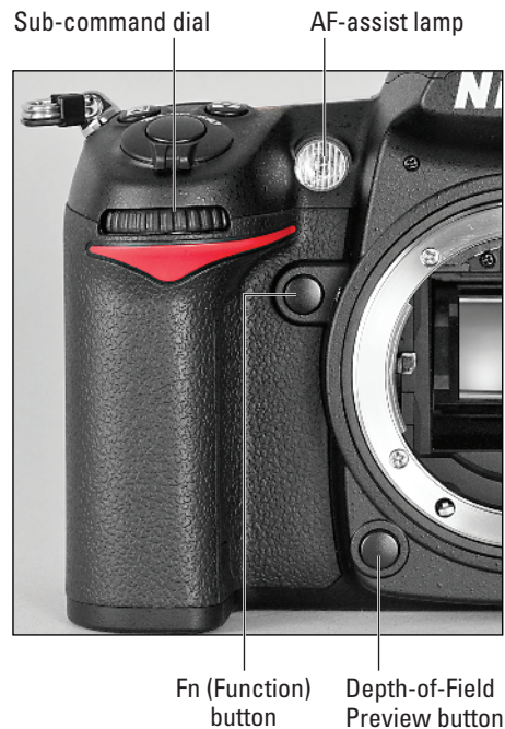
Figure 1-22: You can set the Fn (Function) and Depth-of-Field Preview buttons to perform a variety of operations.
