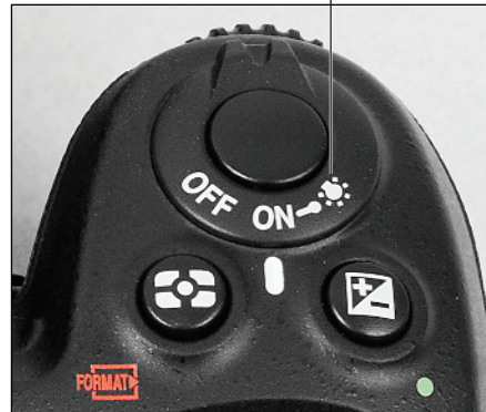
Figure 1-10: Rotate the On/Off switch to the light bulb position to illuminate the Control panel.
