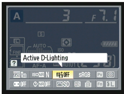
Figure 1-12: Press the Info button while the Information screen is displayed to gain quick access to the settings at the bottom of the screen.
