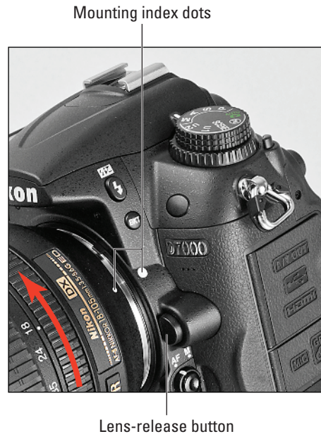
Figure 1-3: When attaching the lens, align the index markers as shown here.
