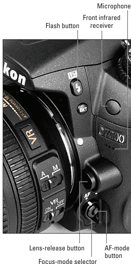
Figure 1-21: Press the Flash button to pop up the built-in flash.
