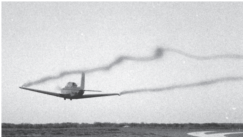
Figure 1.2 Aircraft wingtip vortices. Smoke is introduced at the wingtip to mark the vortex cores. Photograph by W. L. Oberkampf.
