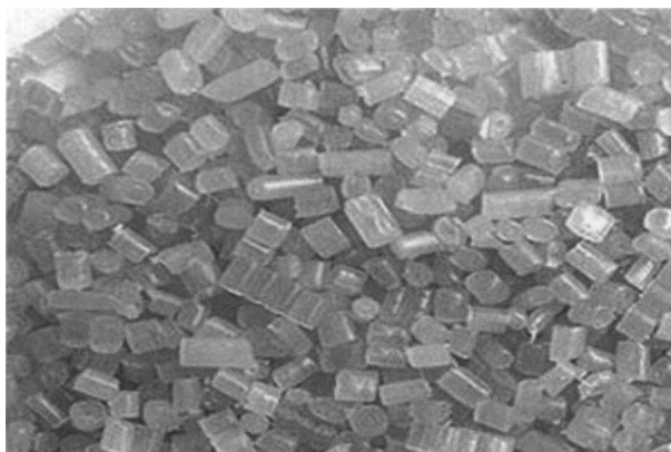
Figure 1.3 Raw polypropylene resin is melted and shaped into pellets of the type shown above. Pelletization increases bulk density, improves handling characteristics and reduces shipping costs. Pellet size is typically ~3 mm (or ~0.1 in). (Reproduced from Introduction to Industrial Polyethylene , with permission of Scrivener Publishing LLC).
