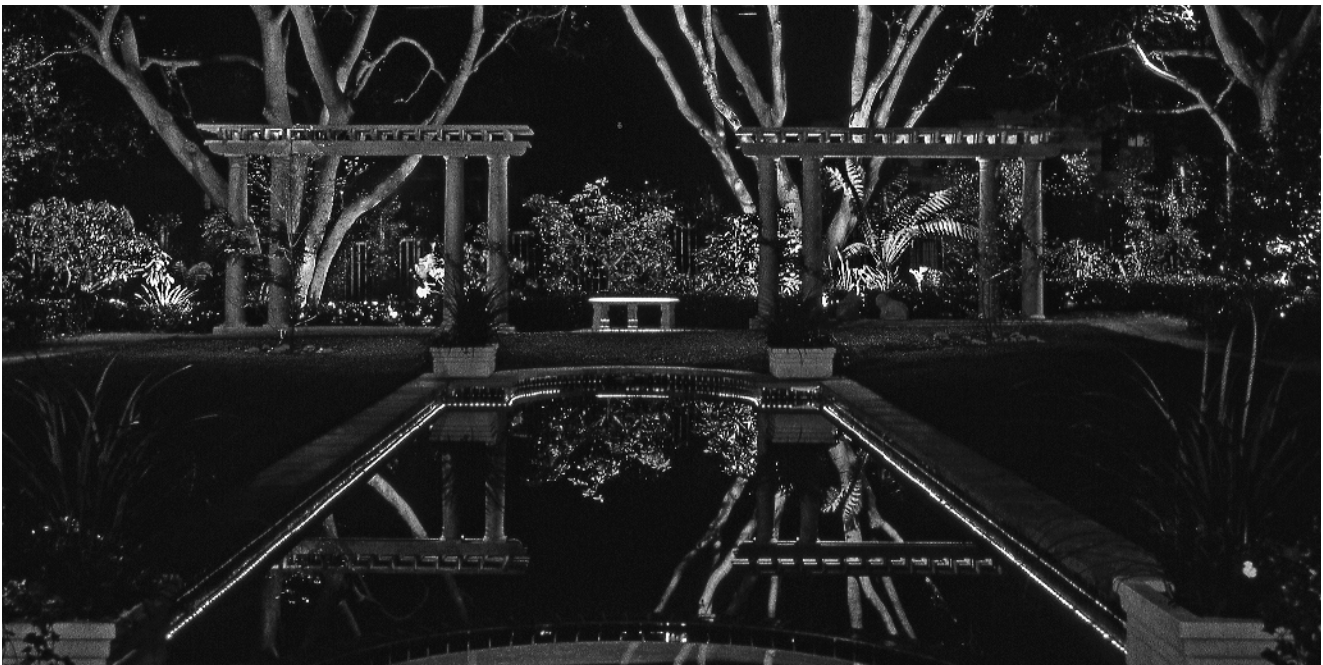
Figure 1.2. Comparing day (Figure 1.2) and the night lighting shows how lighting can transform a landscape. The bench at the end of the pool is the focal point (20 watts in the 1980s); the line of lighting mounted under the pool coping visually expands the garden's depth; and the "ground plane" is lit to the brightest level making the space human-friendly. Lighting Design: Janet Lennox Moyer, MSH Visual Planners; Photograph: Michael McKinley; Landscape Design: Magrane Latker Landscape Design
