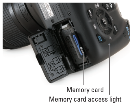
Figure 1-6: Insert the card with the label facing the camera back.
