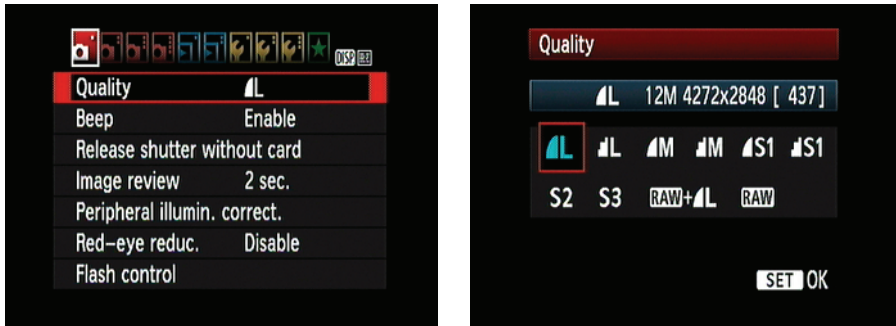
Figure 1-12: Use the cross keys to navigate menus; press Set to access available settings.
