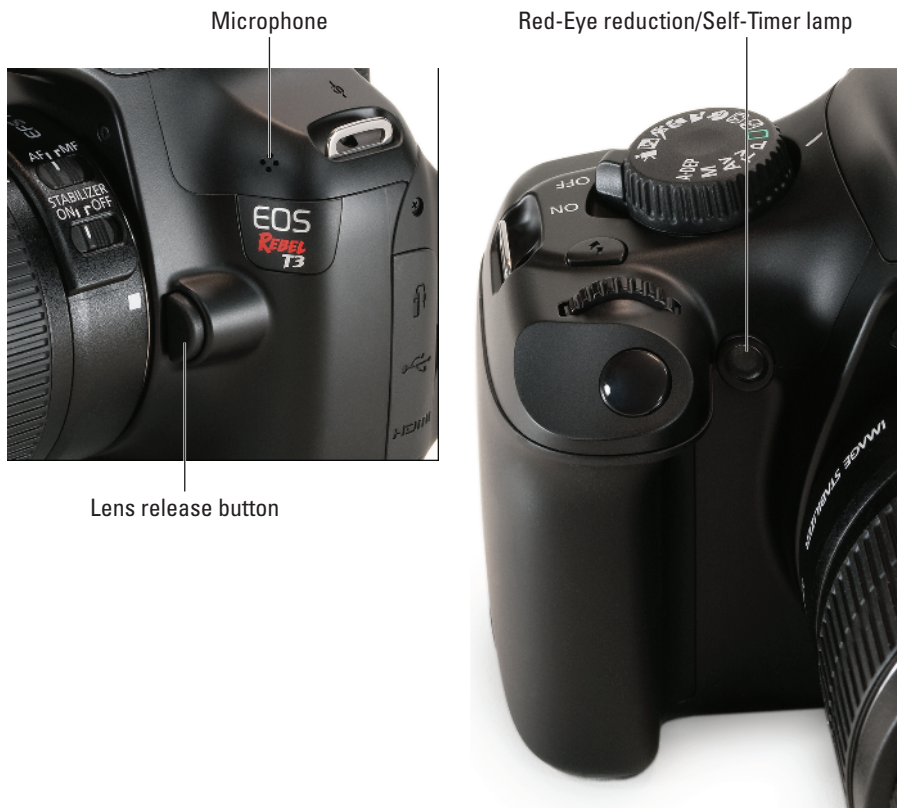
Figure 1-10: Keep your fingers away from the microphone if you're recording a movie with sound.
