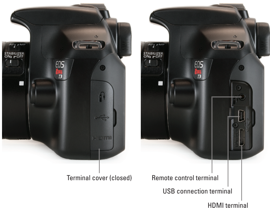
Figure 1-11: This rubber cover conceals connection terminals for connecting the camera to other devices.
