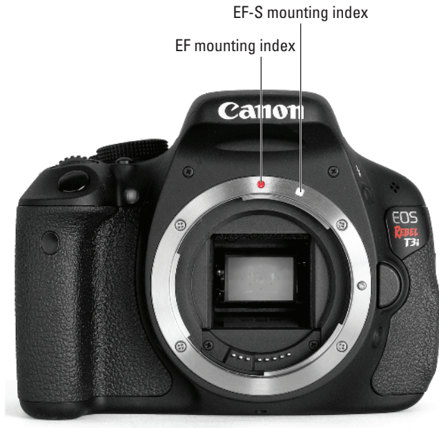
Figure 1-3: Which index marker you should use depends on the lens type.
