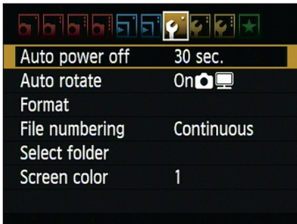
Figure 1-20: Options on Setup Menu 1 deal mainly with basic camera behavior.
