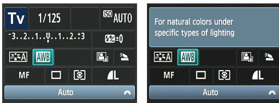
Figure 1-16: Press the Quick Control button to shift to Quick Control mode; the active option appears highlighted.
