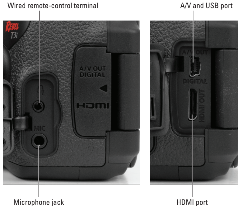
Figure 1-12: These two rubber covers conceal terminals for connecting the camera to other devices.
