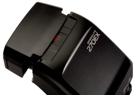
1.18 The Canon Speedlite 270EX Tele-zoom/bounce head
