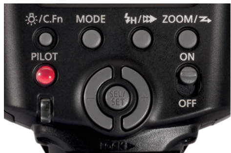
1.16 The 430EX II control panel
