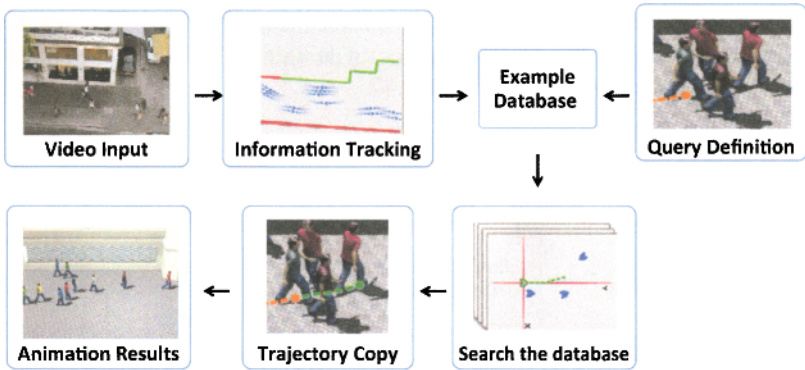
Figure 1.48 Framework of example-based crowd simulation technique. The top row depicts the construction of the database, which takes place during preprocessing: the input video is manually tracked, generating a set of trajectories which are encoded as examples and stored in the database. At runtime (bottom row) the trajectories of the agents are synthesized individually by encoding their surroundings (forming a query) and searching the database for a similar example. The trajectory from the example is copied to the simulated agent.
