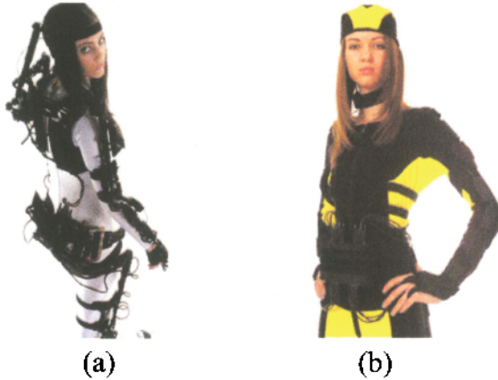
Figure 1.3 (a) Electronic mechanical motion capture system (b) Electromagnetic motion capture system.
