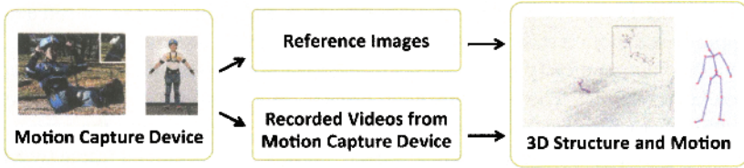
Figure 1.6 A novel motion capture system which captures both relative and global motion in natural environments using cameras mounted on the body.
