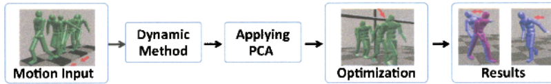
Figure 1.21 The framework of controlling virtual character with a generic class of dynamic responses to small perturbations.
