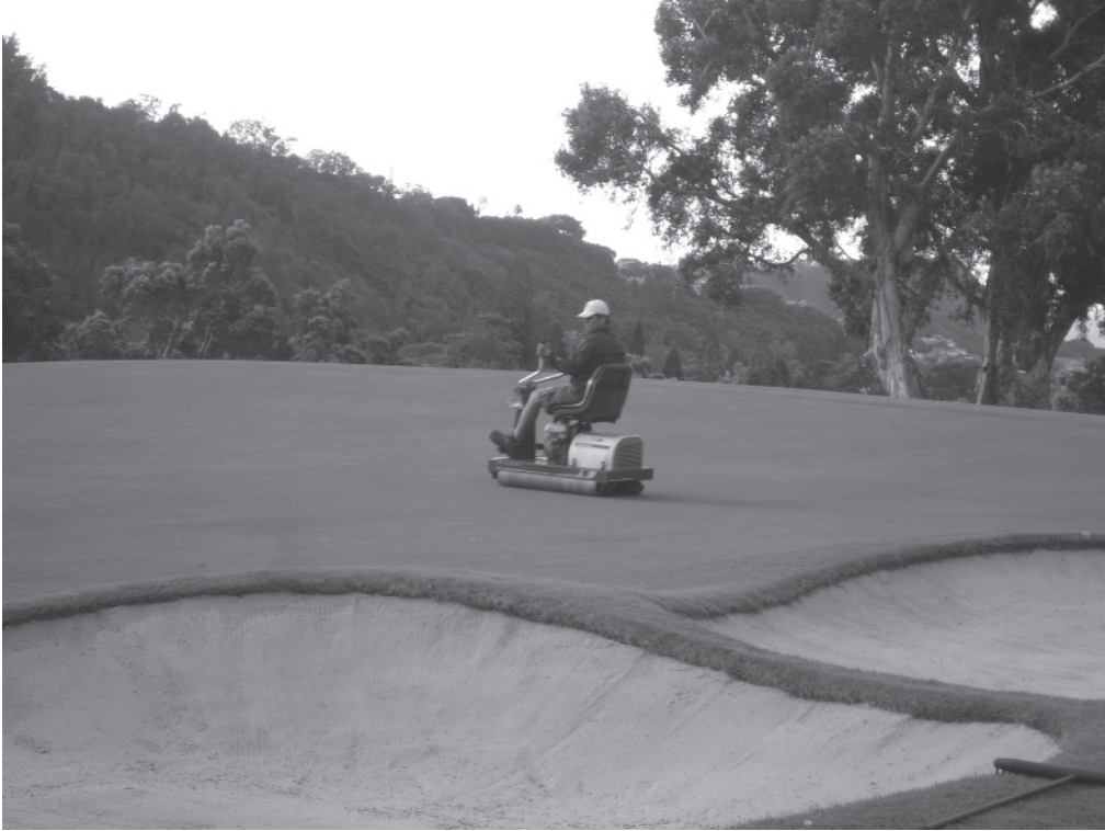
Figure 1.4 A fast-moving greens roller will create a smooth putting surface quickly. (Photo by Curtis Kono, Oahu Country Club.)
