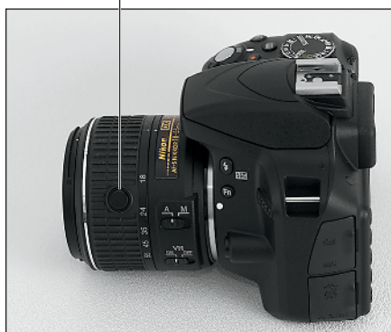
Figure 1-3: Press the lens lock button while rotating the lens barrel to extend and retract the lens.
