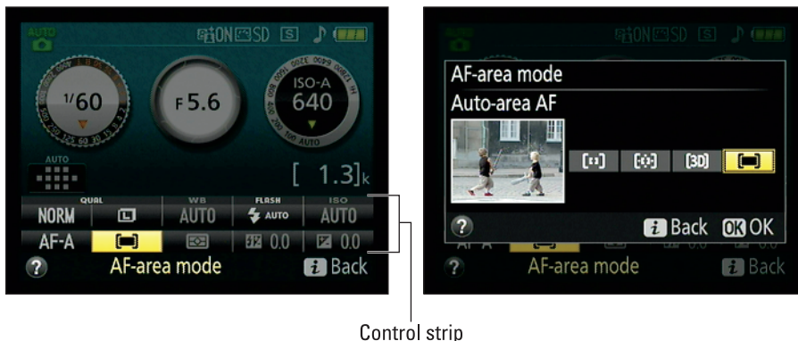
Figure 1-17: Press the i button to activate the control strip (left); highlight the option you want to adjust and press OK to display the available settings (right).
