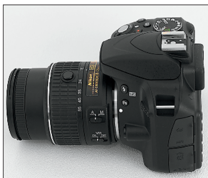
Figure 1-3: Press the lens lock button while rotating the lens barrel to extend and retract the lens.
