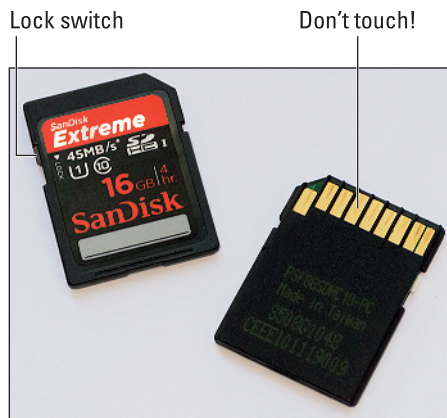
Figure 1-20: Avoid touching the gold contacts on the card.
