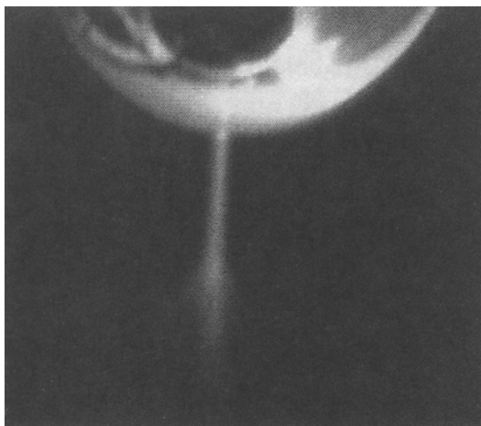
Figure 1.8. Positive brush discharge from negatively charged plastic to grounded sphere (Britton, 1999).
