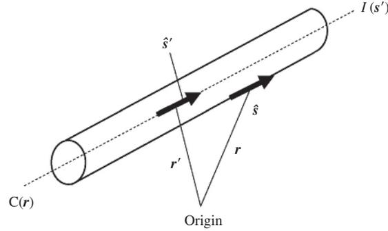
**Figure 1.1** Thin-wire cylindrical segment for method of moment (MoM)-based computation. Current is confined to the wire axis, and the tangential electric field on the surface of the wire is set to zero.
