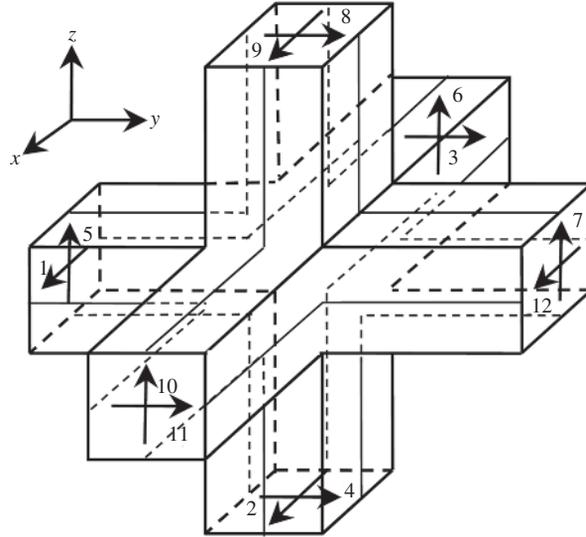
**Figure 1.2** Three-dimensional symmetrical condensed node.
