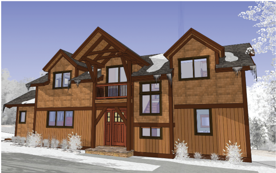
Figure 1.8 Create a winter scene by lightening and desaturating texture images. Timbercreek at Okemo House. Designed by Bensonwood Homes; model built by Michael Brightman
