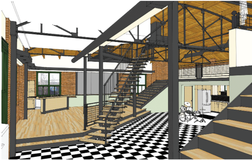
Figure 1.9 SketchUp is as precise as many other CAD programs, precise enough to create as-built 3D models like the one shown. Denver Loft 3D as-built model; space measured and model built by Michael Brightman
