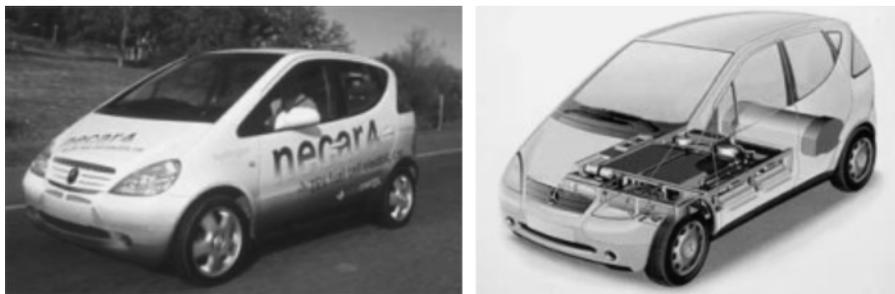
**FIG. 1.2** NECAR4, a fuel cell vehicle with a PEM system operated with liquid  $H_2$  [71].
