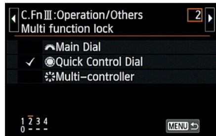
Figure 1-39: This Custom Function determines what control is affected by the Lock switch on the back of the camera.
