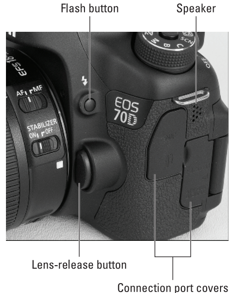
Figure 1-16: Press the Flash button to bring the built-in flash out of hiding.
