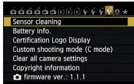
Figure 1-38: You can set the camera back to its default settings by choosing Clear All Camera Settings on Setup Menu 4.
