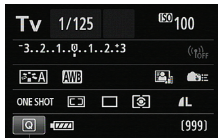
Figure 1-31: To shift to Quick Control mode from the Shooting Settings screen, tap the Q icon or press the Q button.
