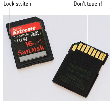
Figure 1-13: Avoid touching the gold contacts on the card.
