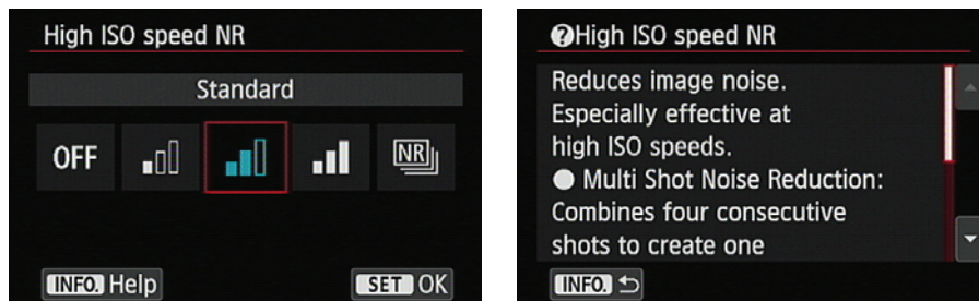
Figure 1-34: If you see the Info/Help icon (left), you can tap the icon or press the Info button to display information about the selected feature (right).
