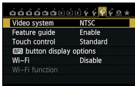
Figure 1-37: Head to Setup Menu 3 to enable or disable the Wi-Fi functions.
