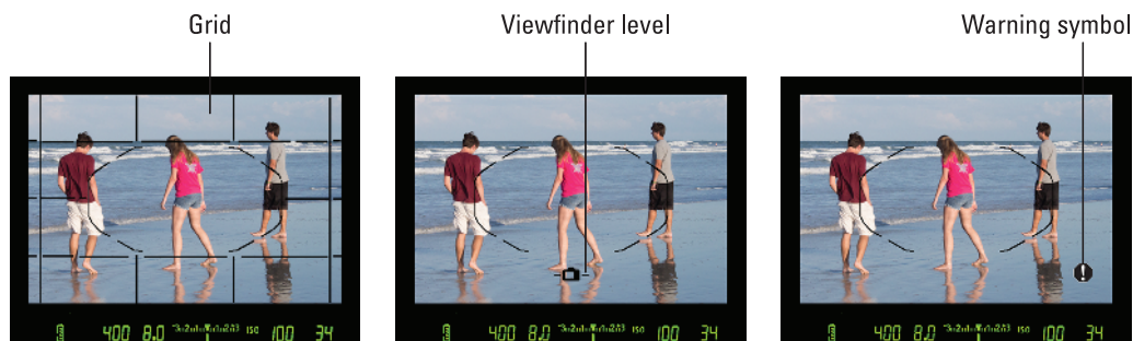
Figure 1-28: You can display a grid (left), an electronic level (center), and feature alert (right) in the viewfinder.
