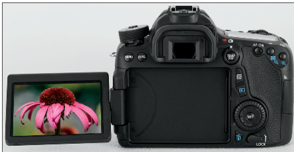
Figure 1-7: You also can unlock the monitor from the body and then rotate the screen to get the best view of things.
