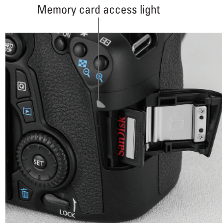
Figure 1-12: Insert the card with the label facing the camera back.
