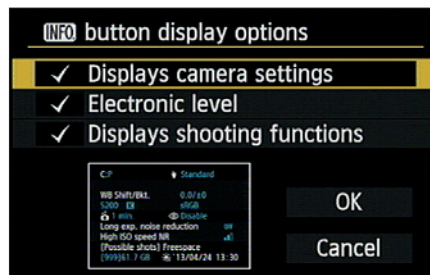
Figure 1-24: Choose which screens the Info button displays during shooting via this menu option.
