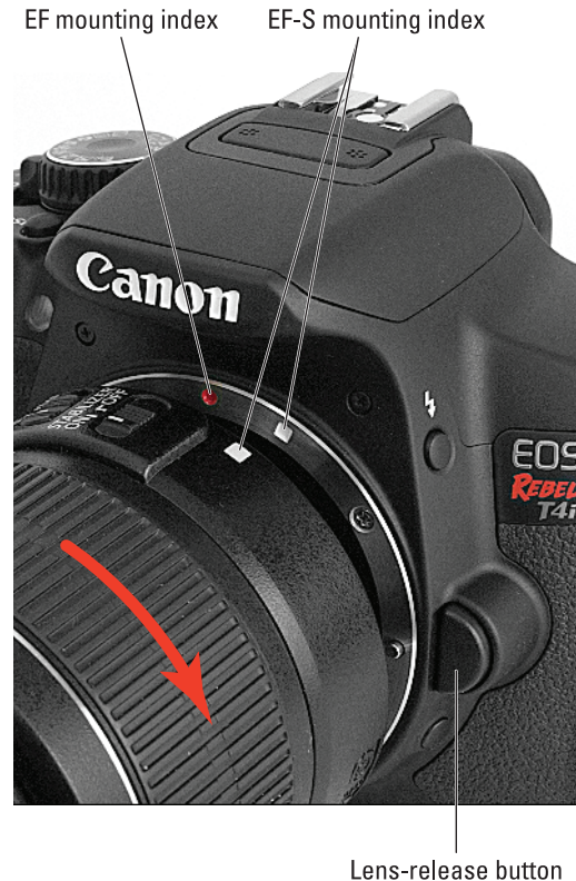
Figure 1-1: Place the lens in the lens mount with the mounting indexes aligned.
