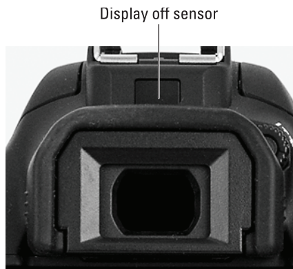
Figure 1-18: The Shooting Information display turns off automatically when the sensor detects your eye covering the viewfinder.
