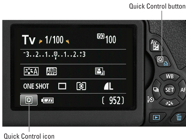
Figure 1-21: To shift to Quick Control mode, tap the Q icon or press the Quick Control button.
