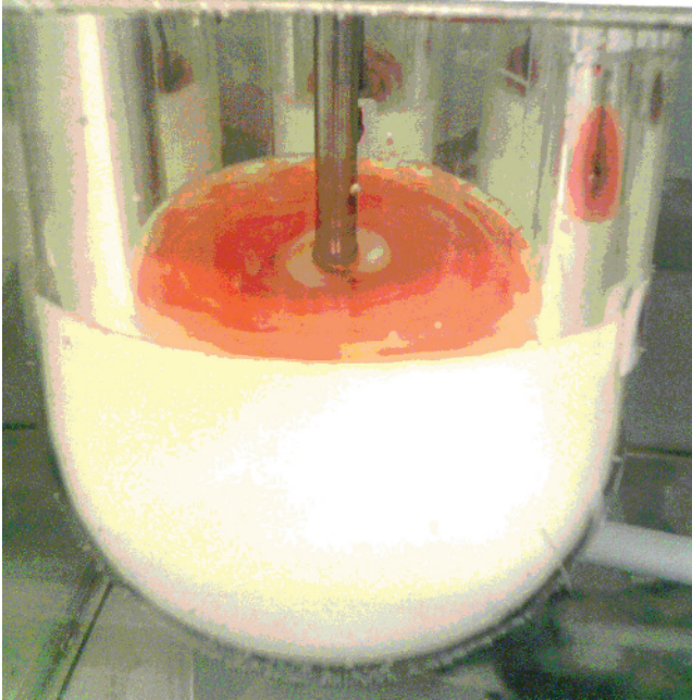
Figure 1.10 Appearance of the lipid formulation of RO-50X in the paddle apparatus after dissolution of the capsule shell. The lipid phase has been colored with Sudan red for visualization.
