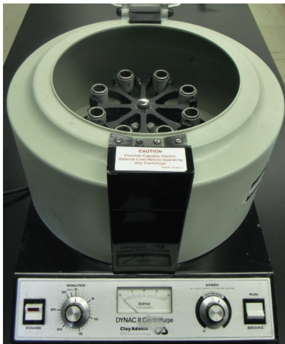
Figure 1.6 Variable angle centrifuge. Buckets swing out horizontally during the centrifugation process.
