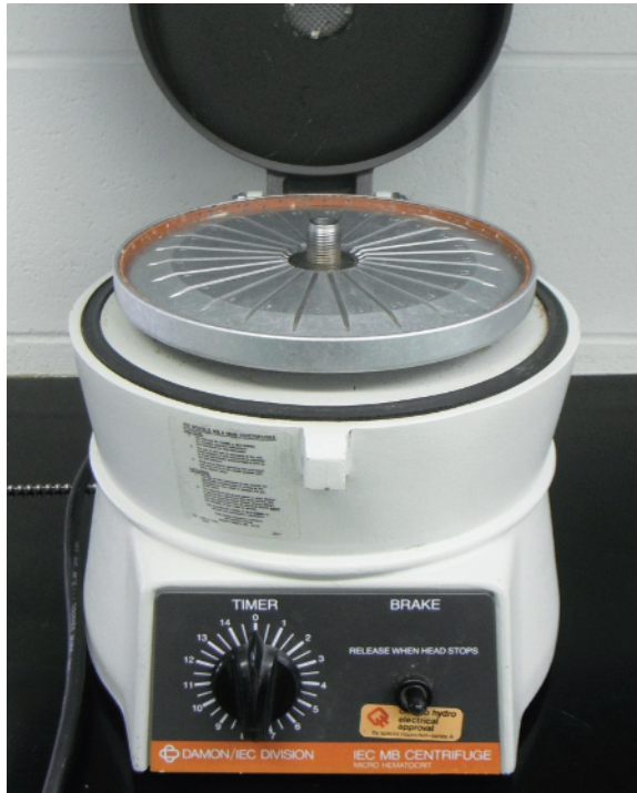
Figure 1.5 Microhematocrit centrifuge. This centrifuge is used for spinning microhematocrit tubes only. It is preset to 10,000 rpm.
