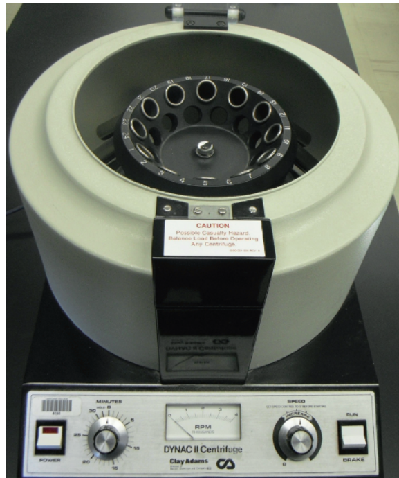
Figure 1.7 Fixed angle centrifuge. Buckets are at a fixed angle (typically about 50°) and do not move during the centrifugation process.
