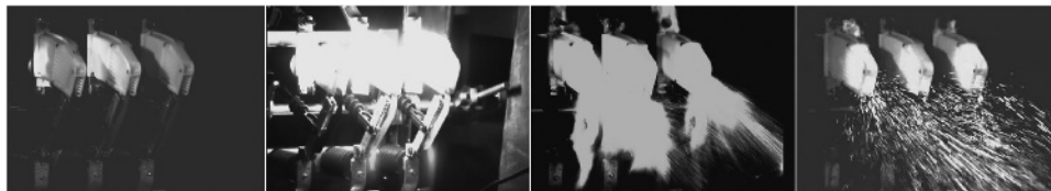
Figure 1.6 Switching arc of a load-break switch interrupting 700 A in a 12 kV test circuit.
