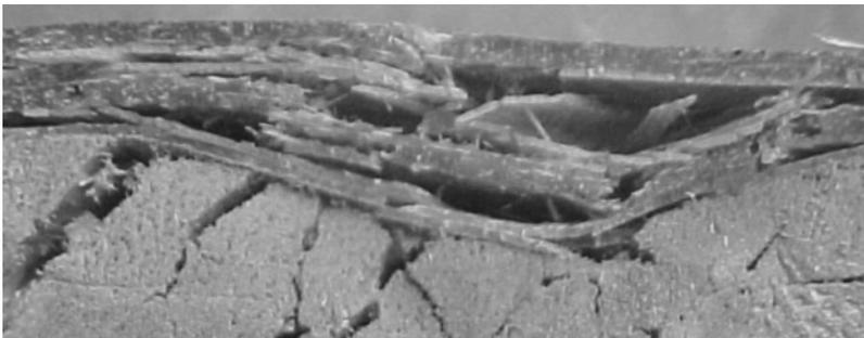
**Figure 1.4** Low velocity impact induced delamination, debonding, and shear fracture in the laminated skin and balsa wood core
