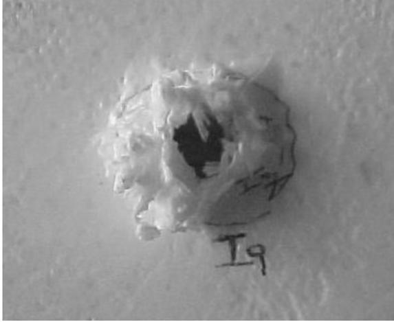
**Figure 1.5** Perforation in a 3-D woven fabric reinforced polymer composite after repeated low velocity impact. *Source:* [39] Reproduced with permission from IOP Publishing
