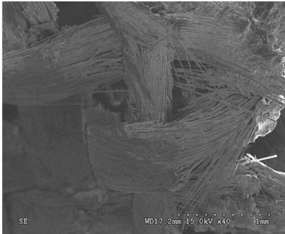
**Figure 1.6** Fracture of fiber tows after repeated low velocity impact. *Source:* [39] Reproduced with permission from IOP Publishing
