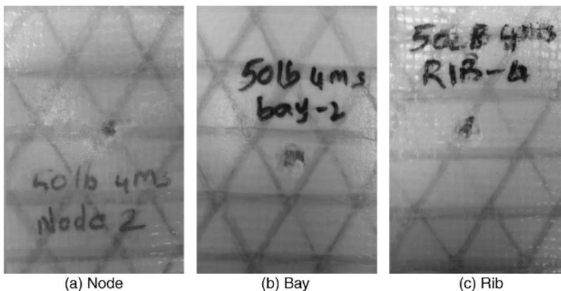
**Figure 1.8** Localized damage in an isogrid stiffened composite subjected to impact energy of 193 J. Source: [19] Reproduced with permission from Elsevier
