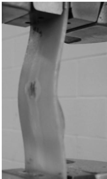
**Figure 1.2** Mixed global and local buckling of a laminate after a moderate velocity impact.
