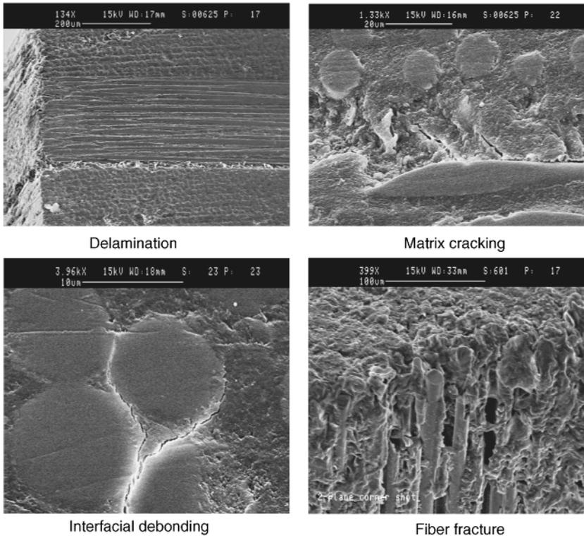
**Figure 1.1** Low velocity impact damages inside a laminate. *Source:* [3] Reproduced with permission from Elsevier
