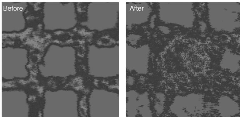
**Figure 1.9** Pre- and post-impact of an orthogrid stiffened composite subjected to an impact energy of 48.8 J at the center of the bay. *Source:* [16] Reproduced with permission from Elsevier
