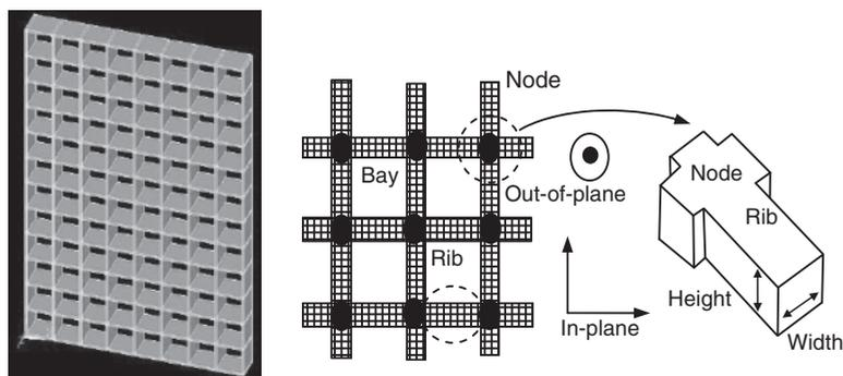
**Figure 1.7** Schematic of an orthogrid.
