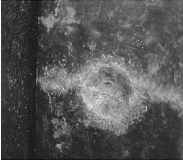
**Figure 1.3** Low velocity impact induced indentation on the sandwich skin
