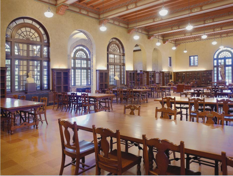
**Figure 1-10** For the grand public reading room, flooring was returned to natural cork to match the original design, low-VOC paints and coatings were specified, and designers also upgraded aging incandescent lighting. *Photograph courtesy of Gensler*
