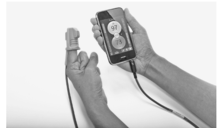
Figure 1-5. The Phone Oximeter ™ checks the level of oxygen saturation in the blood. (Courtesy of LGT Medical)
